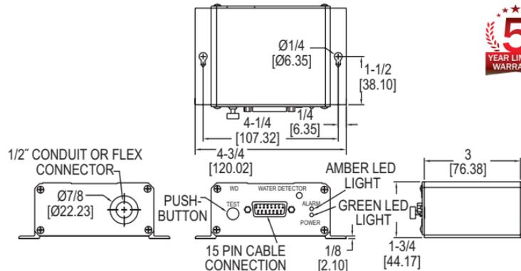
The **Series WD Water Detector and Sensor Tape** is designed for dependable detection of water presence even of low conductive liquids. The water sensing tape attaches to module and if any liquid comes in contact with the tape the resistance is changed and the alarm will be triggered. The sensing tape is 1" wide and can be bought in lengths of 5, 10, 15 and 25' and is powered by 24 VAC or 24-30 VDC.
