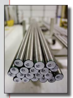
Our drilled barstock thermowells are machined from NACE compliant materials, including 304 and 316 stainless steel, Hastelloy® C276, carbon steel, chrome molybdenum and others. After production, we polish our thermowells to a minimum surface finish of 32  $\mu$ in  $R_a$  and mark them to ensure material traceability.
