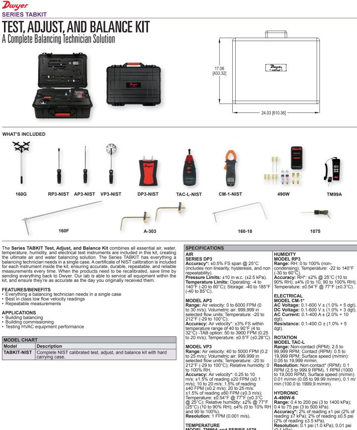
M/s), 10 to 20 m/s, 15% of reading ±40 FPM (±0.2 m/s); 20 to 25 m/s; ±1.5% of reading ±60 FPM (±0.3 m/s); Temperature: ±0.54°F @ 77°F (±0.3°C @ 25°C); Relative humidity: ±2% @ 77°F (25°C) (10 to 90% RH); ±4% (0 to 10% RH and 90 to 100%). Resolution: 1 FPM (0.001 m/s).
