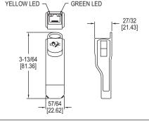
The Model MN-1 Mini-Node™ Communication Signal Converter is a low cost device that converts half duplex RS-485 serial communications signals into a signal that can be read by any computer with a USB port. The integral USB connector and RJ-45 connector reduces set up time by eliminating extra wiring. The Model MN-1 is powered via the USB connection which eliminates the need for an external power source. The compact size is great for field installation, control panels, and lab testing.
