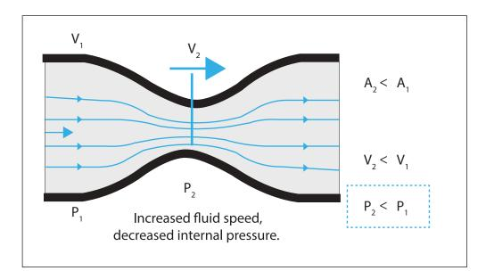
As the fluid enters the upstream part of the Venturi Tube, the flow contracts and is accelerated due to the gradual decrease in cross-sectional area, creating a pressure loss.
